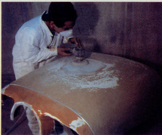
Primer and paint go on with wheels and flight controls removed (top). The engine upgrade required the moving of the oil access door—another patch to sand (above). Inspection panels and fairings get painted separately (below).
